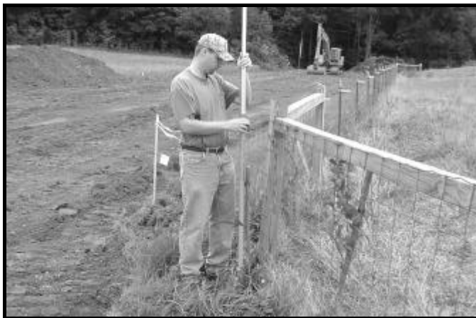
Jeremy Huggler, part of the District's technical staff, conducting a land survey. The data gathered is used in a Computer Assisted Design program (AutoCad) to create engineering drawings. Contractors then construct conservation practices such as grassed waterways, ponds or wetlands, all of which protect water quality.
